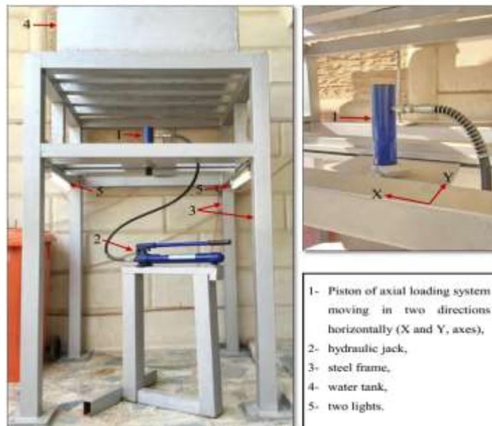
*Plate 4: Steel loading frame and loading system.*
