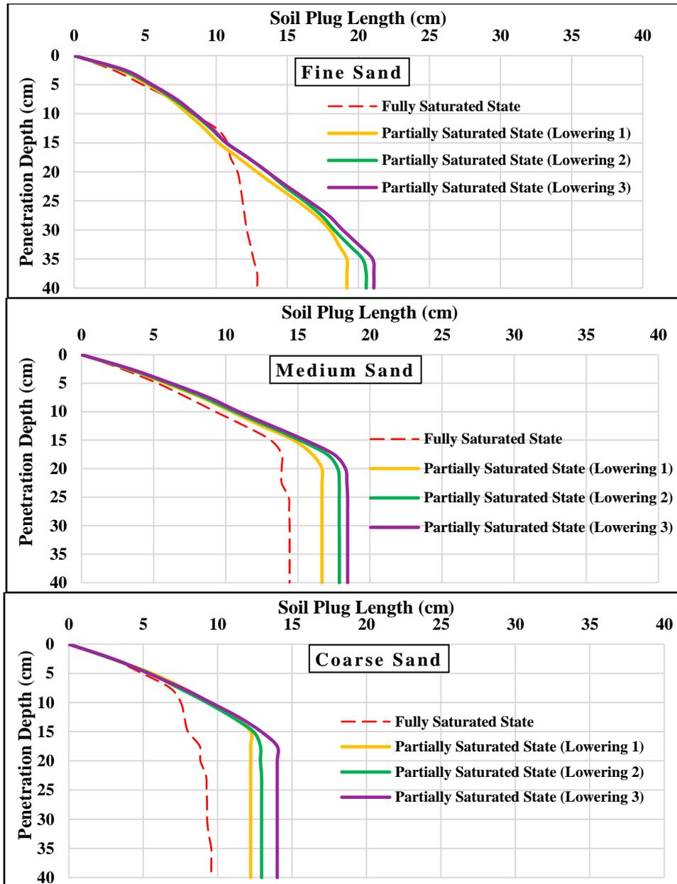
Figure 8: Variation of Soil Plug Length with pile penetration depth at different grain size distribution of soils and saturation conditions for pipe pile of 3.0cm diameter.
