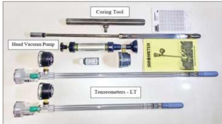
*Plate 3: Low tension-Tensiometers used with their accessories.*
