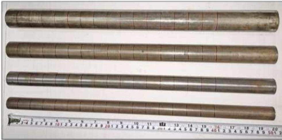
*Plate 1: Pipe piles models.*
